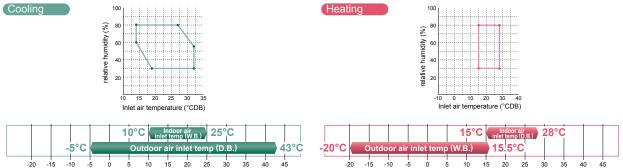
By controlling the air volume of the outdoor unit fan, operation is available even when the outdoor temperature is -5°C for cooling and -20°C for heating.
