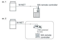
\*When a PAR-31MAAE is connected to a group, no other MA remote controllers can be connected to the same group.
