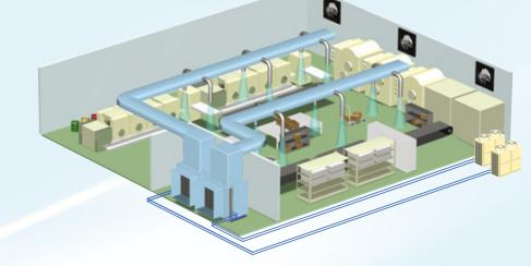
\*1 Fresh air intake type indoor units supply pretreated outside air into the room. This type of units are not designed to handle internal thermal load. Use other types of air conditioning units that are capable of handling internal thermal load in combination with the Fresh Air Intake type units.
